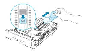
2 After inserting paper into the tray, slide in the guide until it lightly touches the end of the paper stack.
